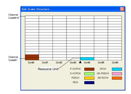
Figure 3.1.6-1 Sub-frame Structure Screen (Link=DL)
